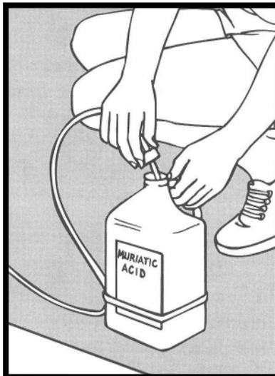
2. Place rubber band around lower  $\frac{1}{3}$  of bottle (see picture). Screw vent cap on gallon container of diluted muriatic acid (5:1 recommended). Use chlorine for organic stains.
