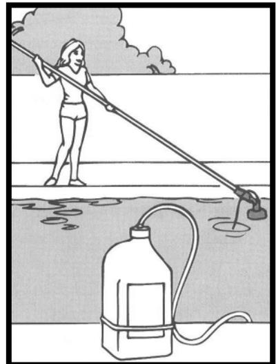
4. Submerge vinyl hose tubing and applicator in pool, stretching tube out all the way to remove coils.
